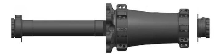
Unscrew the preload adjuster dust cap with a Torx 8.
