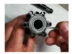
**STEP 19** Reinstall the bearing holder ring.
