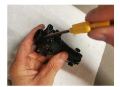
**STEP 2** Unscrew the preload adjuster dust cap.
