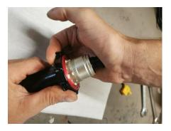
Tighten both ends with a 17mm spanner. Do not overtighten! Maximum 10Nm.
