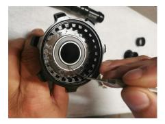
**STEP 13** Remove the bearing seal.
