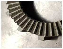
**Floating ring:** check all teeth edges are still sharp, do not use it anymore if there is a jagged cuts on the teeth. The squares of the splines are 2.8mm (when new). Always check if the contact surfaces of the splines are still square and flat. They should not be rounded!
