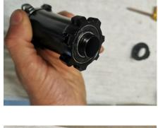
If you have the experience: remove the seal, clean the bearing and apply SKF bearing grease. If needed change the bearing.
