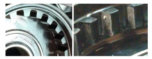
**Rear hub housing:** the squares are 2.6mm (when new). Do not use them anymore if they are less than 2mm or extremely worn and/or with irregular shapes! There are two possible positions of the floating ring inside the rear hub housing. Please do not place a new floating ring arbitrarily. You should mark the first position with a waterproof marker and use the second unused spline position in the rear hub housing.
