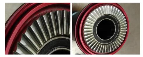
**Freehub ratchet:** small wear is normal. Check if all the teeth edges are still sharp. Do not use it anymore if there is a jagged cut on the edge of the teeth. If more excessive wear is present, this could be because there is to much play on the axle and the freehub ratchet floats too much. This causes more damage than intended.
